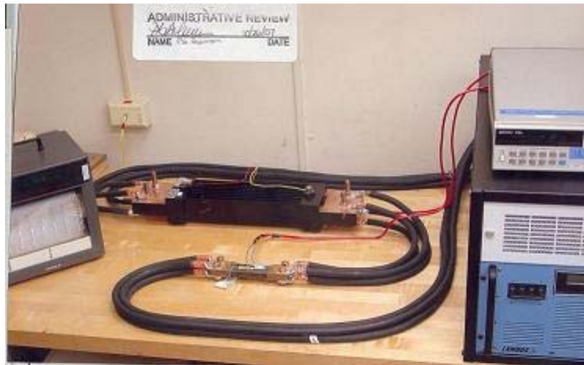
Figure 2. Shunt comparison system – note proper lead wire connection and orientation
