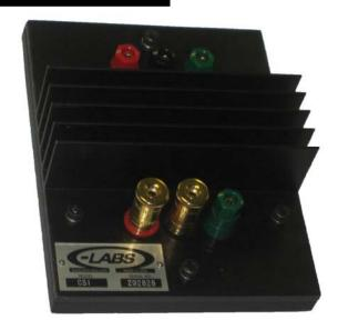
Connection is via gold plated binding posts, which accept wire, banana plugs and spades. Connection errors common to other shunts are minimized by the internal bus structure.
